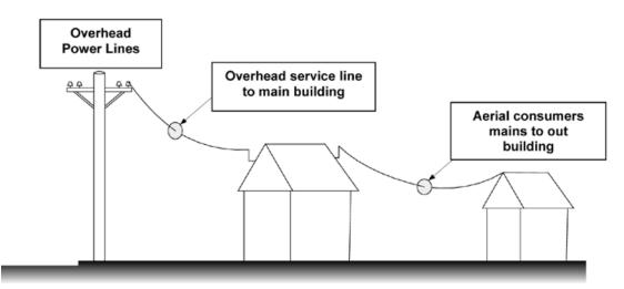
Figure 14 – Low Voltage Overhead Service Lines
