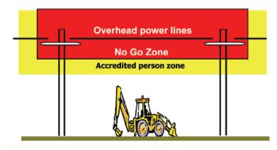
Mobile plant including cranes, excavators, EWPs, earth moving machinery, tipper trucks and concrete placing booms whose design envelope is within the approach distances specified in Table 1 must be controlled by safe systems of work as described in this chapter.
