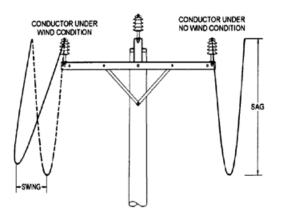
Figure 2: Illustration of overhead power line 'sag or swing'
