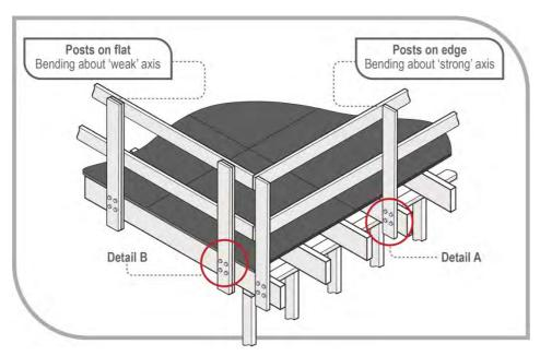
Figure 8a Timber guard rails - posts subject to bending about their weak and strong axes
