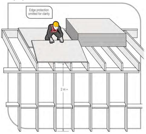
Figure 15 Laying sheet flooring at upper level
