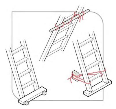
Figure 12 Examples of effectively securing a ladder
