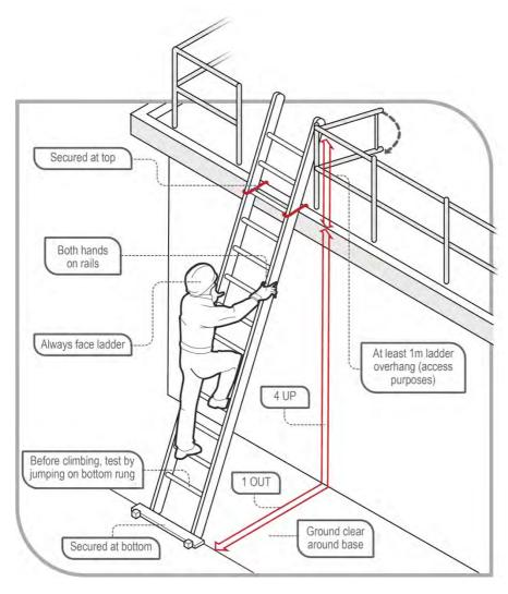
Figure 13 Example of acceptable ladder use
