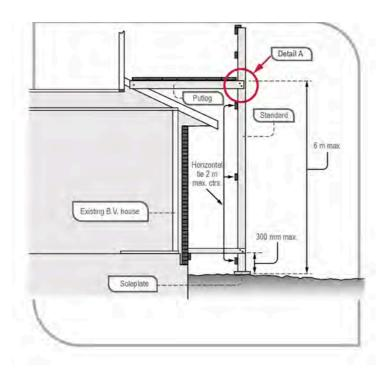
Figure 30 Timber scaffold (single pole - high first lift)
