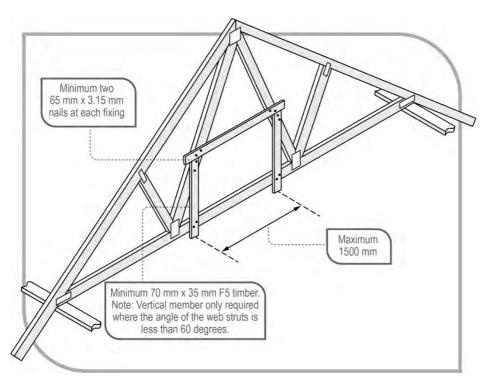
Figure 23 Suggested method of fixing temporary waling plate
