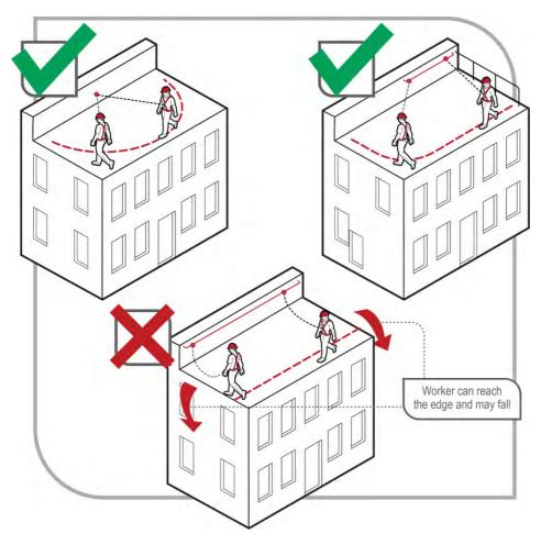
Figure 9 Restraint technique options
