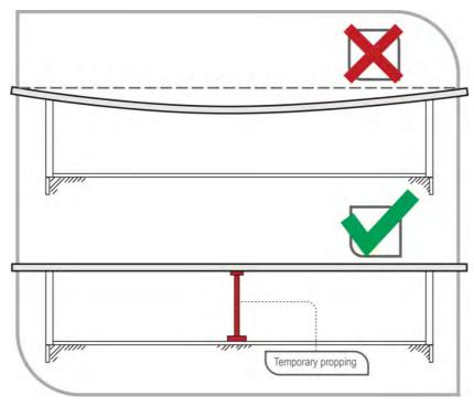
Figure 21 Method of supporting long trusses
