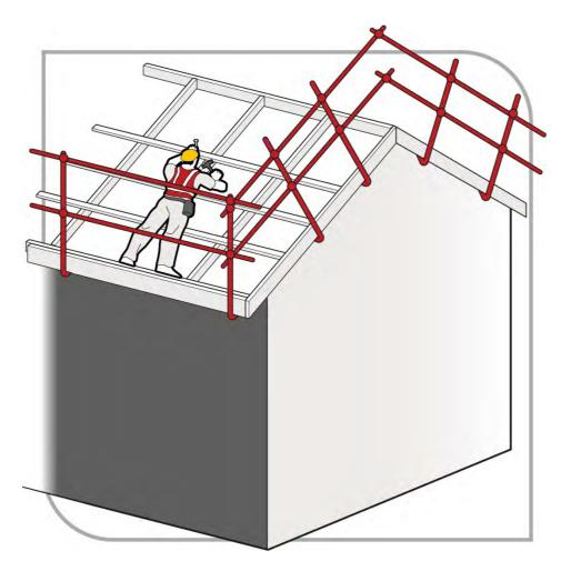
Figure 27 Fixing roof battens to trusses
