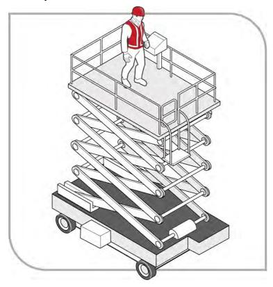
Figure 6 Scissor lift elevating work platform
