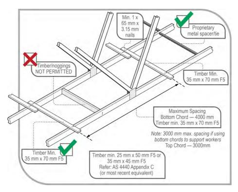
Figure 26 Temporary bracing/ties to bottom chord of trusses. Note: Bracing to top chord similar
