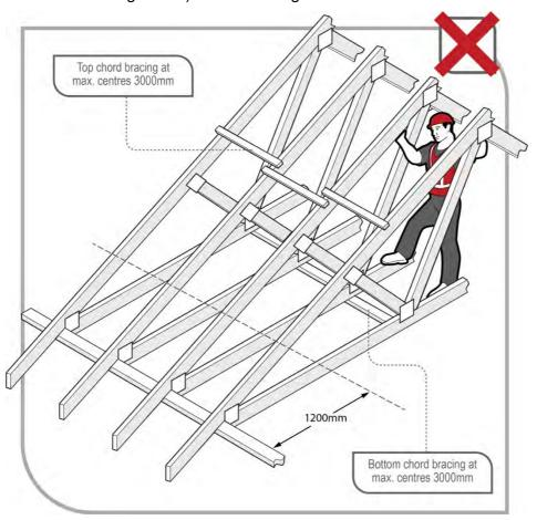
Figure 22 No go zone for persons erecting trusses
