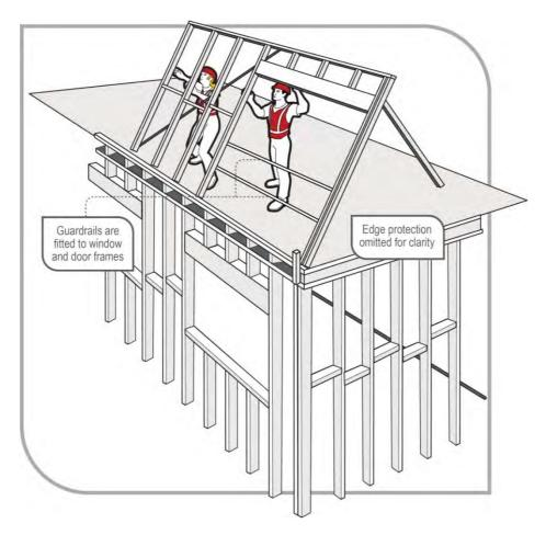
Figure 20 Erecting upper level wall frames
