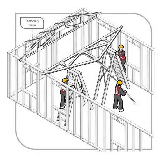
Figure 25 Recommended method of manually standing trusses with a high apex
