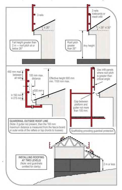
Figure 28 Guardrail systems for roofing work
