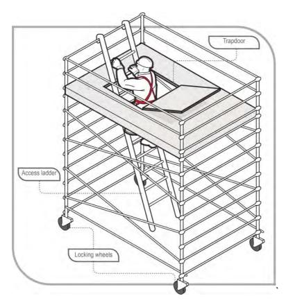
Figure 3 Mobile scaffold with access ladder
