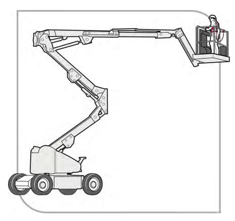
Figure 7 Boom-type elevating work platform
