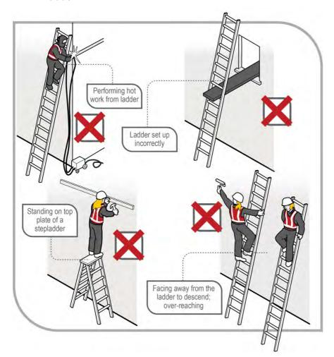
Figure 14 Examples of unsafe ladder use
