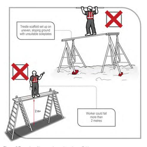
Figure 5 Examples of incorrectly used trestle scaffolds
