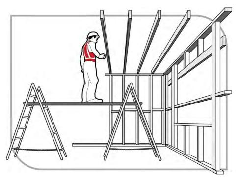
Figure 18 Installing ceiling or upper level floor joists
