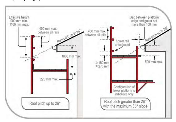
Figure 29 Catch platforms for roofing work
