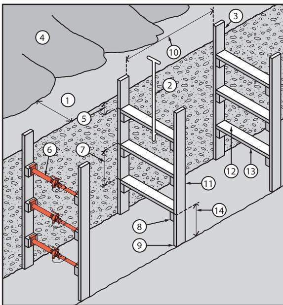
1. Spoil heap at least 1000mm clear of excavation allows access along the side of the trench top and prevents material from the heap rolling into the trench.
