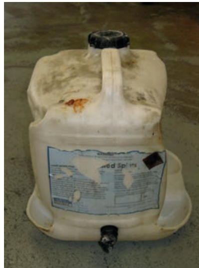
Flame damage to a container of methylated spirits
