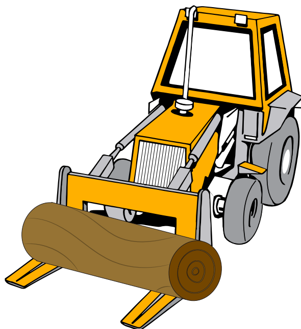
Figure 2: Log Loader fitted with a log beak (grab) that has the capacity to secure logs onto the tines.
