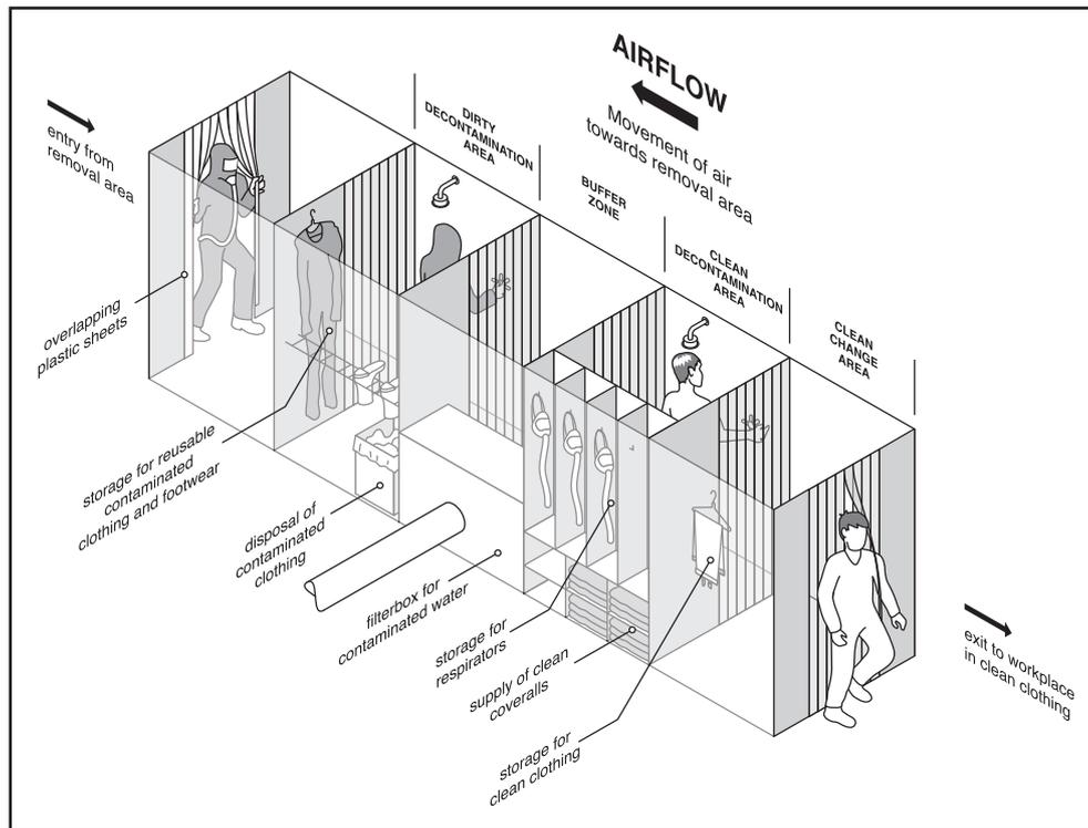
The decontamination unit should be immediately adjacent to and directly connected with the enclosed removal work area. It should be located as far away as practicable from workplace facilities such as and lunch rooms
