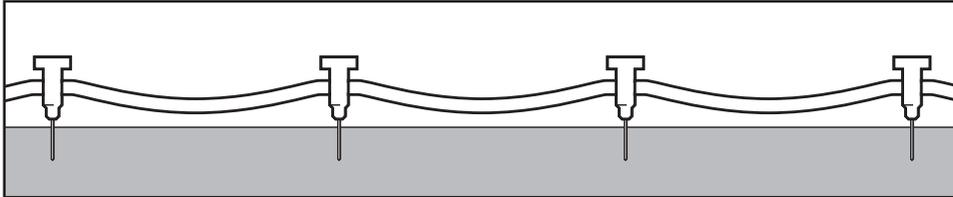
The asbestos is soaked by the introduction of water or other wetting agents through an appropriate applicator that consists of an injection head with numerous side holes or outlets through which the water or wetting agent is fed to the asbestos.
