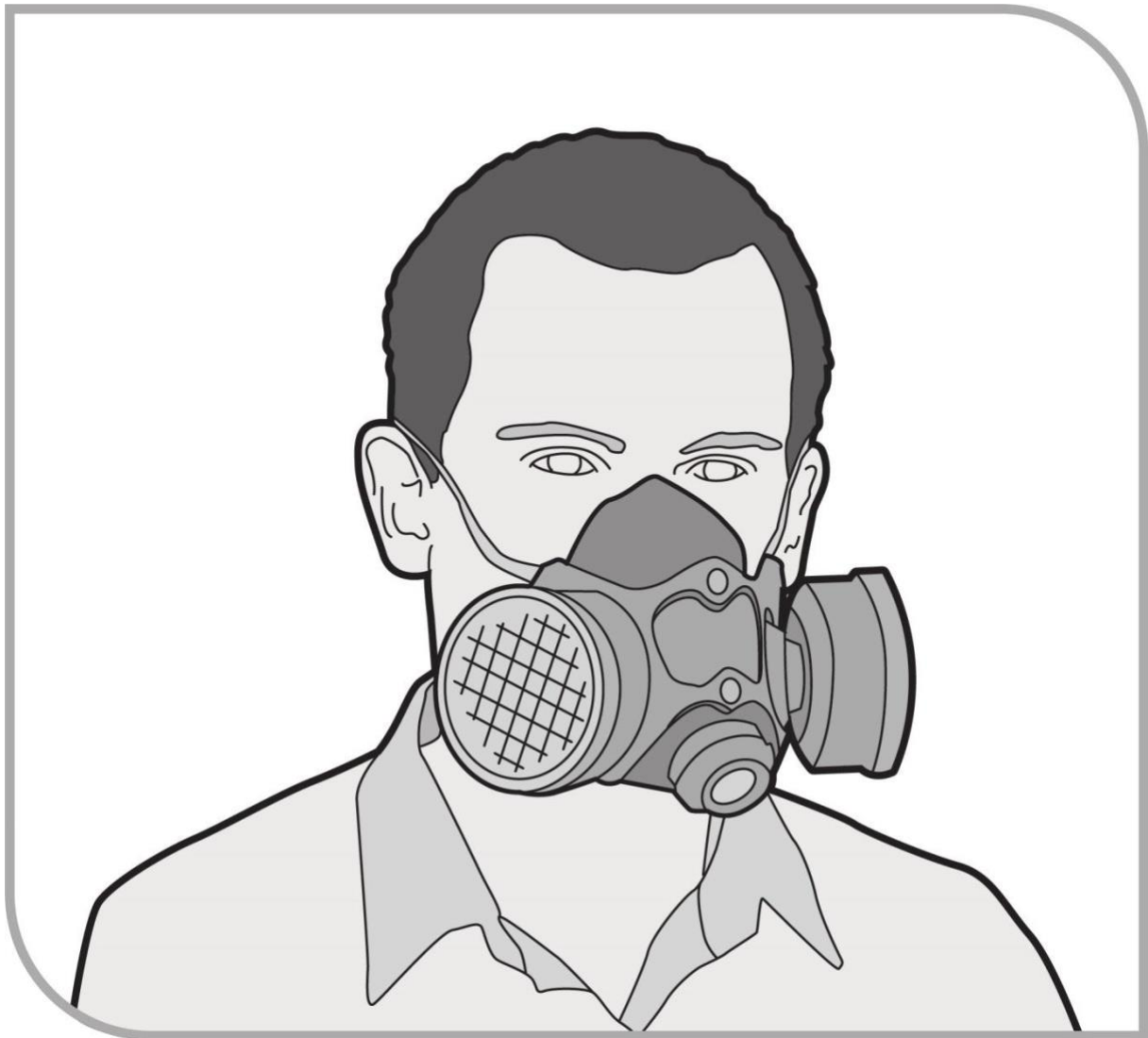
Figure 10 Half-face particulate filter (cartridge) respirator
