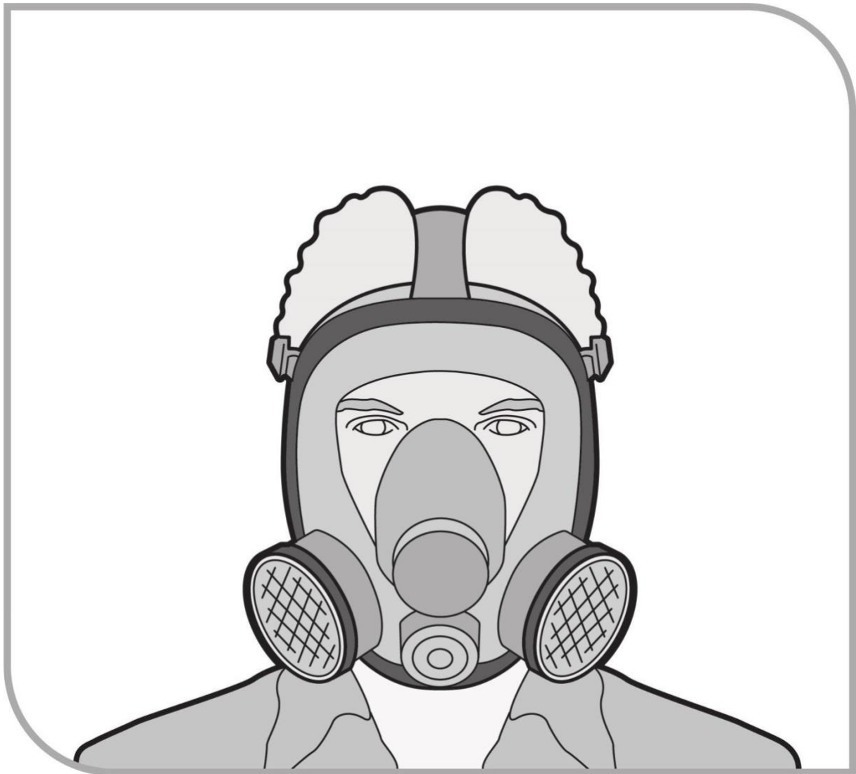
Figure 12 Full-face, particulate filter (cartridge) respirator
