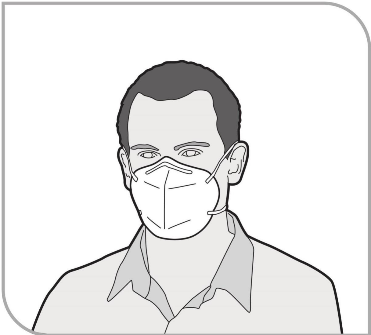
Figure 9 Disposable, half-face particulate respirator
