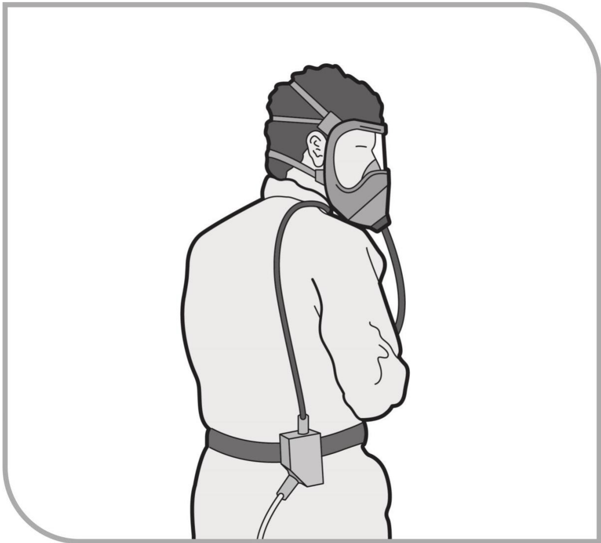
Figure 14 Full-face, positive pressure demand air-line respirator
