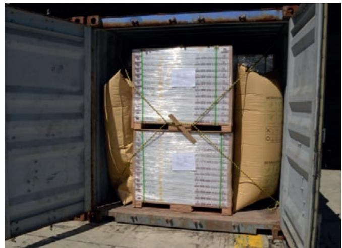
Figure 4: Bulky items packed using crates, wrapping, dunnage bags and strapping.
