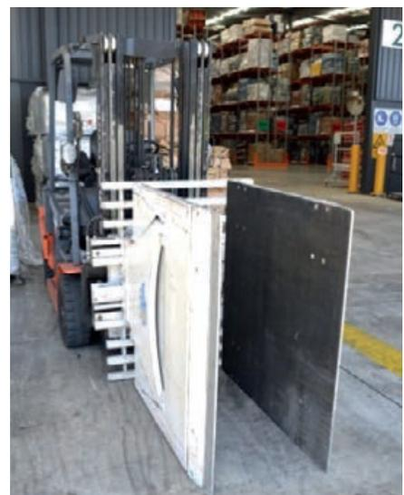
Figure 7: Using suitable equipment to unload such as a fork lift truck with grabs.
