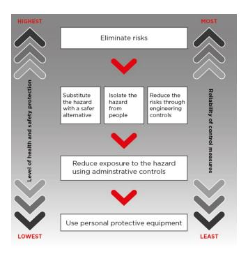
Figure 2 The hierarchy of control measures
