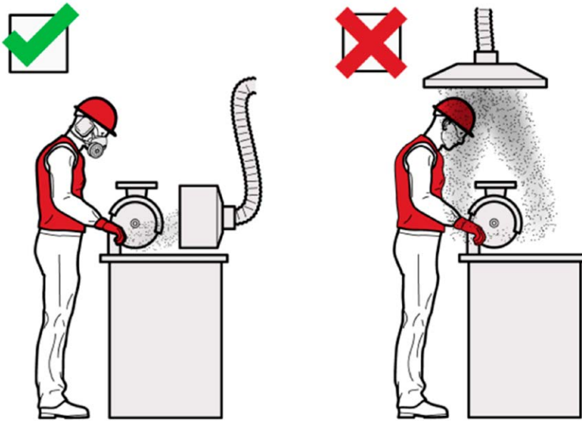
Figure 6: Examples of using local exhaust ventilation
