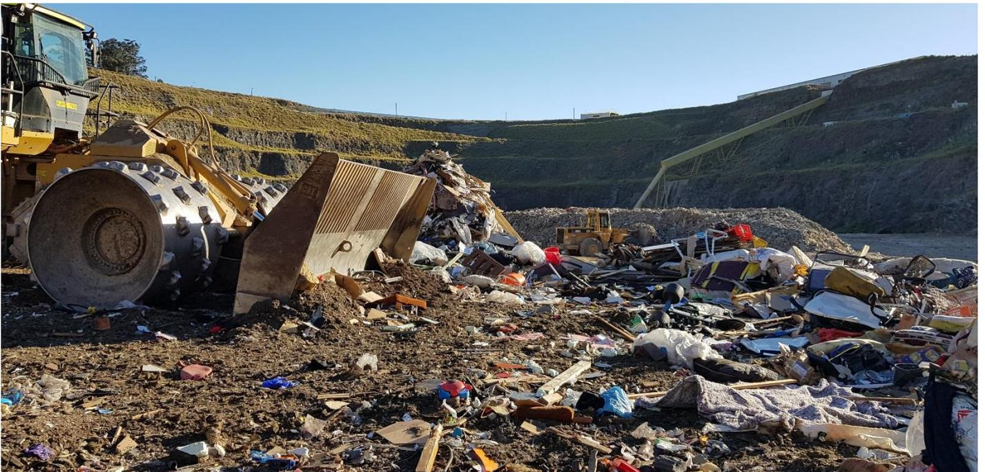
A heavy industrial landfill compactor in the open pit of the waste management facility in Eastern Creek.
