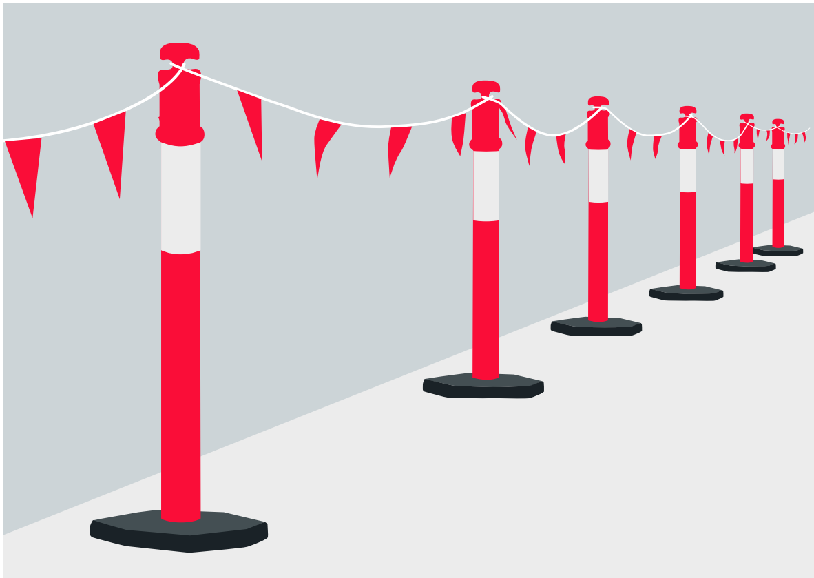
Figure 5: Example of bollards and bunting barrier.
