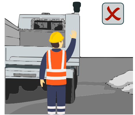
Figure 10 – The wrong place for the spotter to stand. The mirror is out of sight of the spotter and driver does not have a clear view of the spotter.
