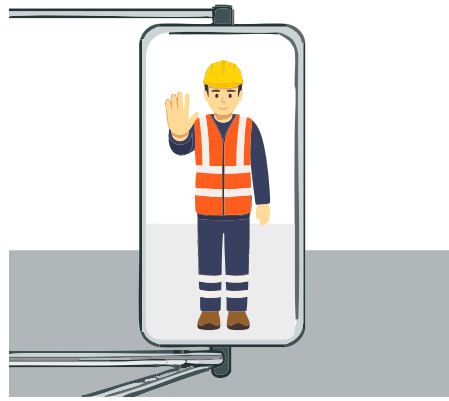
Figure 9 – The view the driver should have of the spotter.
