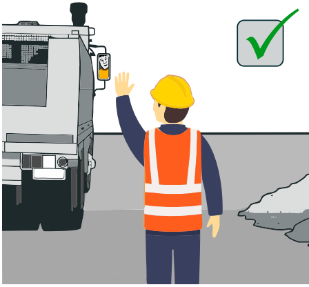
Figure 8 – The correct place for a spotter to stand. The spotter can see the driver and driver has a clear view of the spotter in the mirror.
