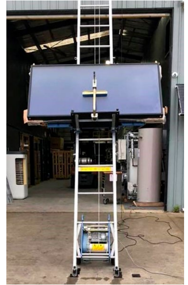
Image 14: Example of a panel lifter
