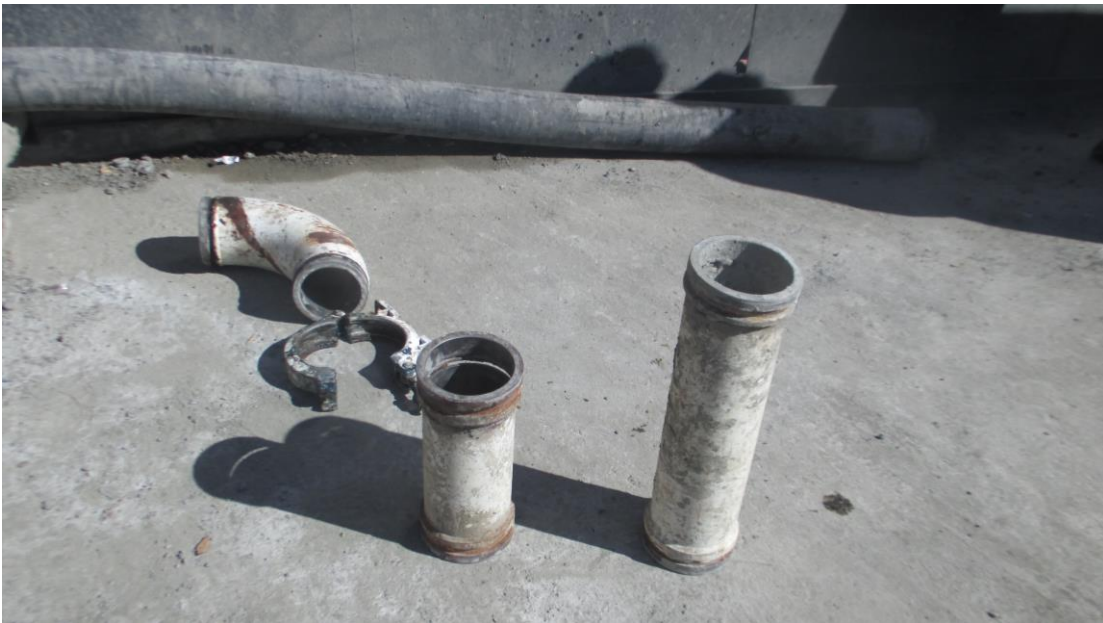
Image of the rubber end (discharge) hose, coupling, elbow and two pump line components.
