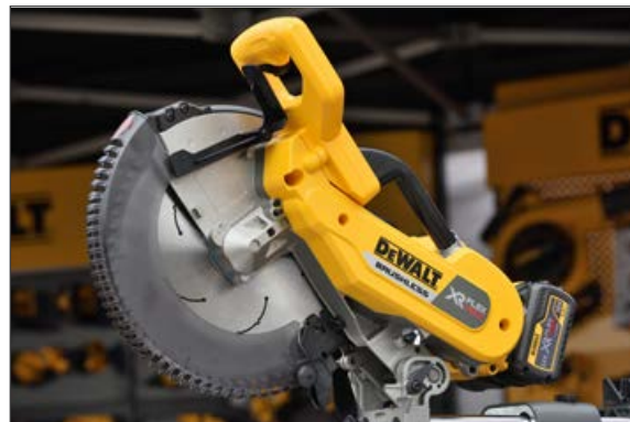
Drop saw with a self-closing guard
