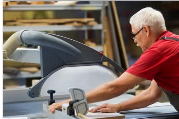
Adjustable top guard with integrated dust extractor
