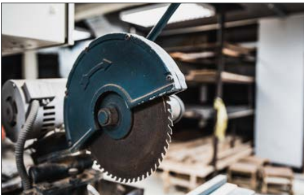
Drop saw without a self-closing guard
