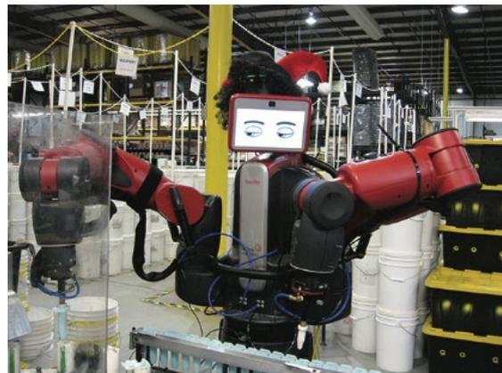
Figure 11: Example of collaborative robot appearance (Sauppé & Mutlu, 2015)
