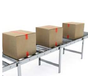
Movable conveyors or electric walkie-stackers to move finished goods to despatch area.
