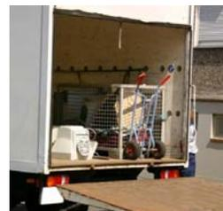
Tailgate lifter to lower and unload cabinets on site.
