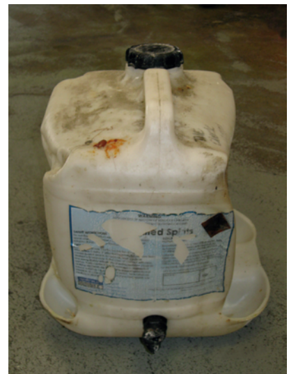
Flame damage to a container of methylated spirits
