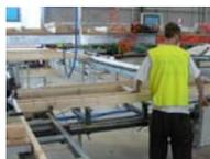
Roller conveyor to move timber to assembly area.
