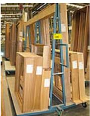
A-frame trolley to transport window frames.
