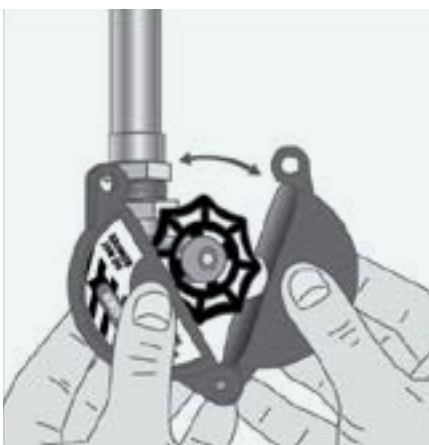
Picture 2. Locking out isolation points, such as this valve, prevents the isolation point from being reactivated.
