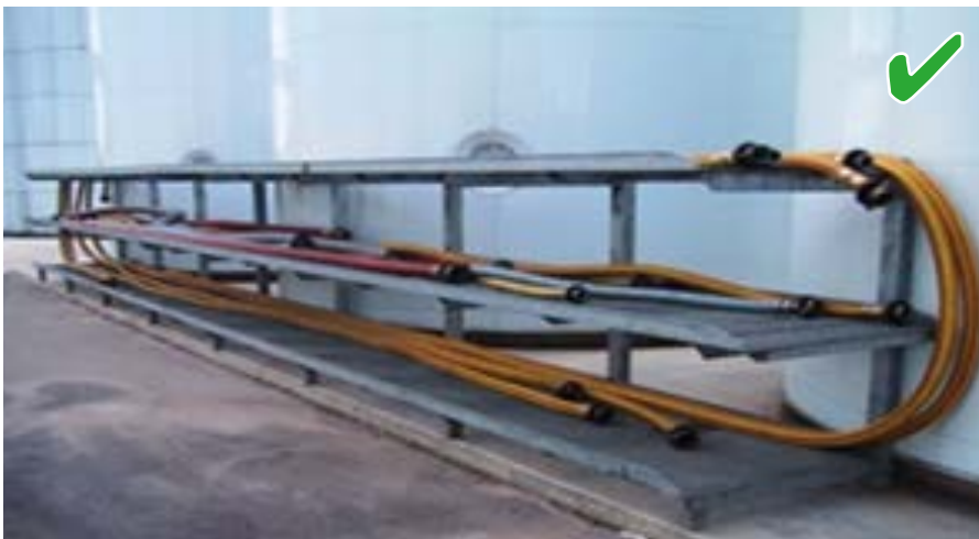
A rack used to store hoses, prevent trip hazards and damage while not in use.
