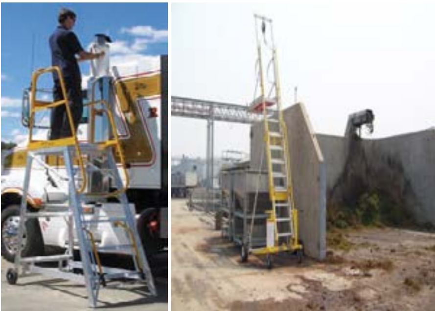
Examples of platform ladders that provide a stable work platform.
