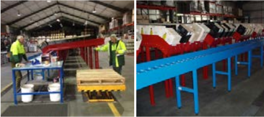
Use of an automated scissor lifts table and manual conveyor for pick, pack and dispatch tasks.
