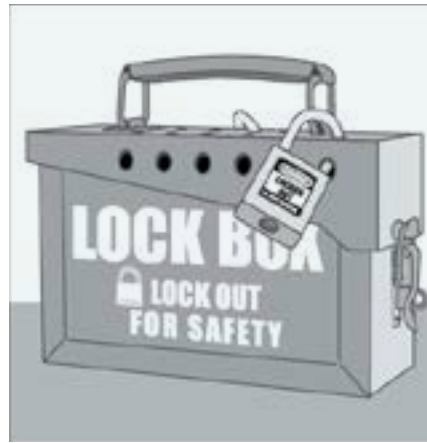
Picture 4. A lock box avoids multiple locks at each point.
