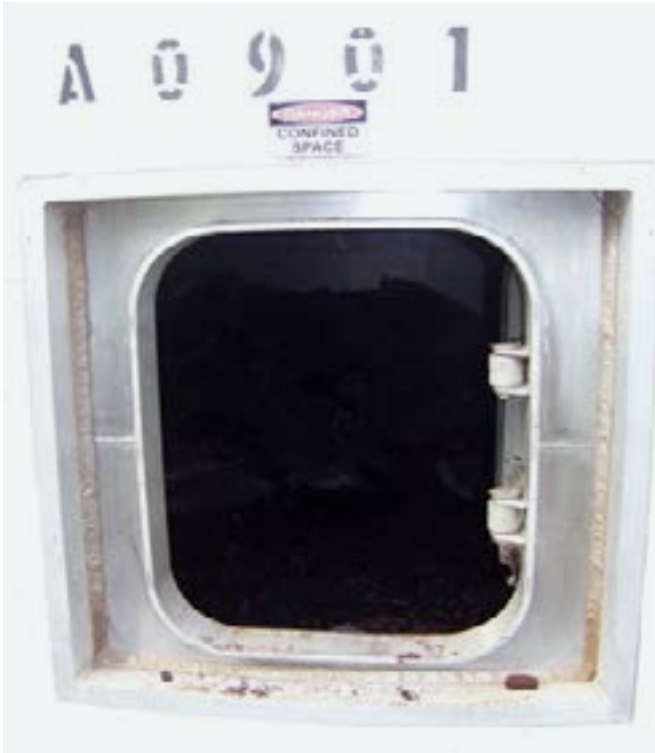
Wine tank identified with confined space danger warning sign.
