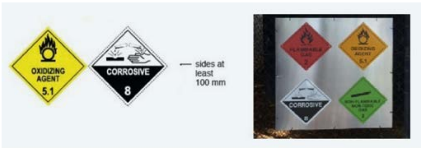
Figure 3 – Example placards for a storage location for hazardous chemicals in packages
