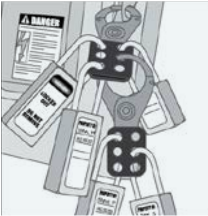
Picture 3. A lock is attached for each worker performing maintenance or non-production tasks.
