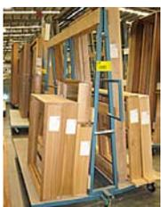
A-frame trolley to transport window frames.
