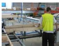
Roller conveyor to move timber to assembly area.
