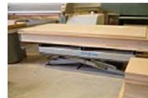
Scissor lifts and air tables to move wood to cutting area.
