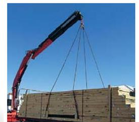
Hoists and hiab cranes to load finished frames and trusses on to trucks
