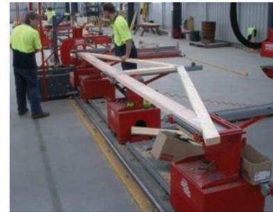
Use mechanical aids, eg a tilt bench, to transfer timber frame from work bench to trolley to reduce heavy lifting.
