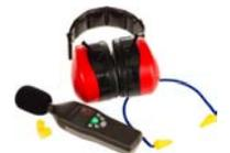
Noise monitors, signage and hearing protection – eg ear muffs to assess and reduce exposure to noise.
